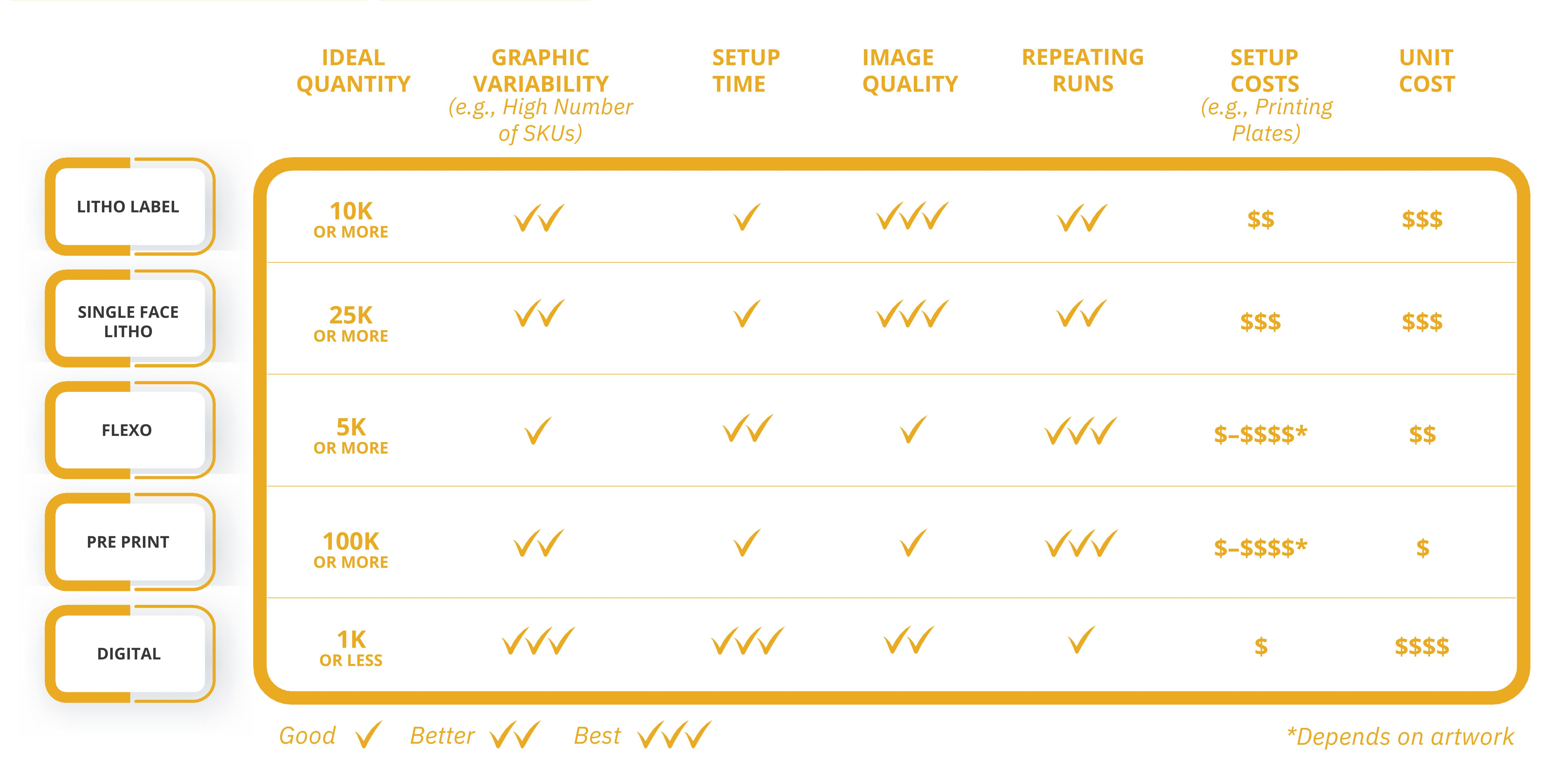
The finished package may incorporate a mix of printing methods for the best of both worlds. For example, a floor display which routinely uses the same base and tray might be printed 1-color flexo, with a digitally printed header that is frequently updated for special promotions or seasonal campaigns.
